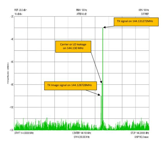
In this example the values are the same, in the real practice the IQ+ XT will have a Carrier suppression in the order of -55dB and a TX Image rejection of -50dB ( with software correction the TX Image rejection will be around -80dB)
