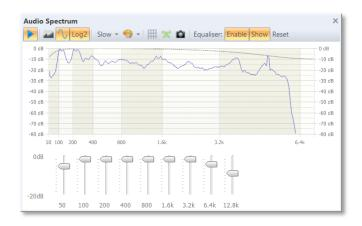
When you select the Show option the equaliser sliders are displayed, the slider range is 20dB. Graphical equalisers are implemented via a series of Biquad IIR filters, one filter per slider.
