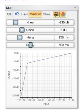
Automatic gain control (AGC) is an adaptive system found in many electronic devices. The average output signal level is fed back to adjust the gain to an appropriate level for a range of input signal levels. For example, without AGC the sound emitted from an AM radio receiver would vary to an extreme extent from a weak to a strong signal; the AGC effectively reduces the volume if the signal is strong and raises it when it is weaker. (From Wikipedia, the free encyclopedia.)
