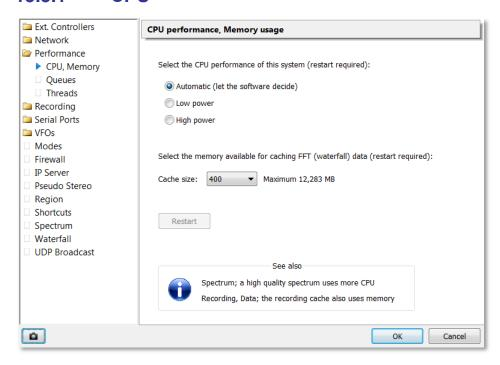
This software is designed to run on anything from a 1.6GHz ATOM processor to the latest i7. When a lower-powered system is used it is necessary to reduce the processing. Normally you let the software decide whether it is running on a low or high-power system; here you can override this setting.
