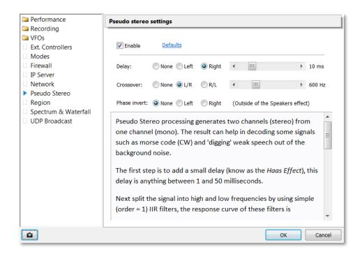
Pseudo Stereo processing generates two channels (stereo) from one channel (mono). The result can help in decoding some signals such as Morse code (CW) and 'digging' weak speech out of the background noise.
