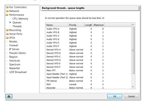
This diagnostic page shows the background thread unprocessed queue sizes (length). If the background threads are not running properly the queue sizes will increase.
