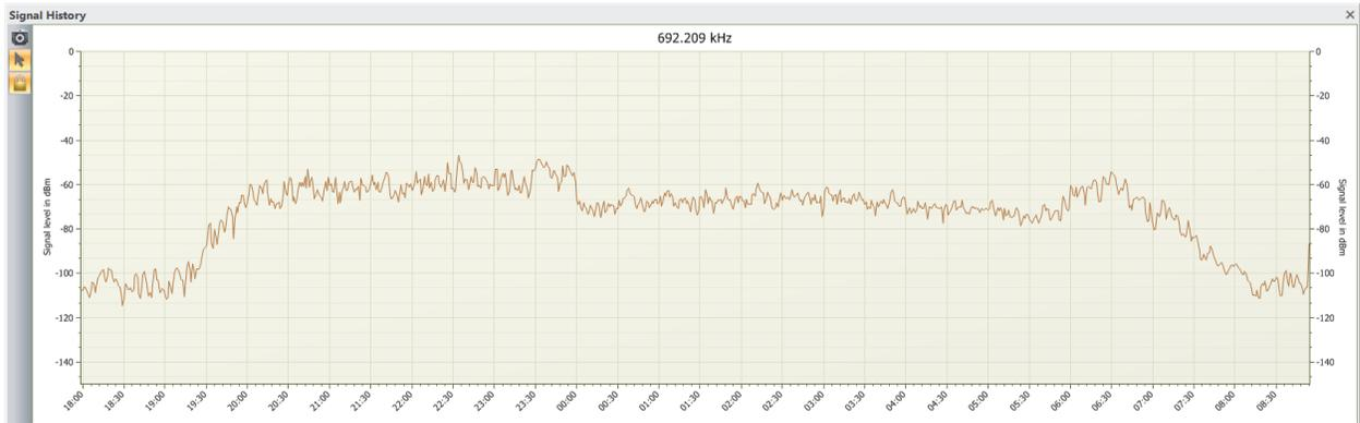
This is a very simple but at the same time useful tool which displays the signal level for the selected frequency over the entire analysis time range. To select the frequency of interest you must first make sure that the mouse is configured to select the signal history frequency, to do this click the mouse pointer button in the signal history toolbar.
