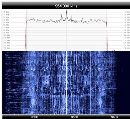
This waterfall shows the signal being passed to the demodulator. You can drag the filter by clicking either of the two vertical filter bars with the left mouse button.
